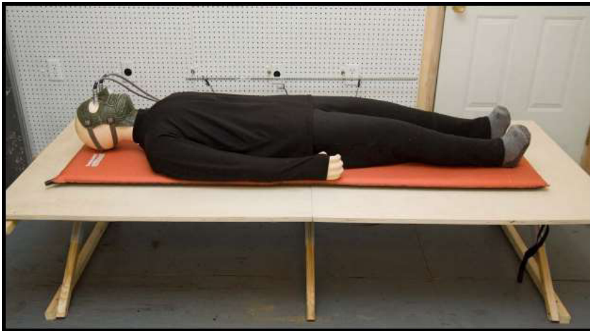
Figure 2. Manikin dressed in the facemask, thermal underwear, and socks on top of the pad and board
